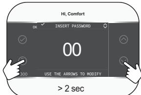
Use the and buttons to set the desired password (INSTALLER - 18 or SERVICE).
